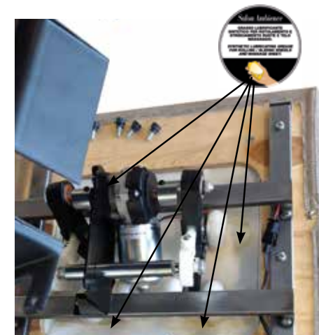
5. Remove the casing and lubricate the PVC back cloth of the massage
